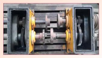
**FZG Gear Test Rig**
