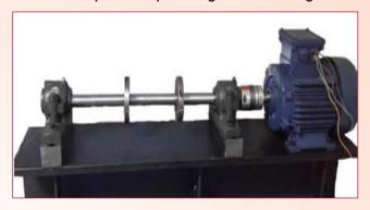
**Bearing Fault Detector Test Rig**
