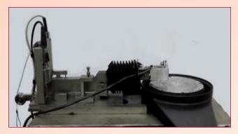
Pin on Disc Tribometer
