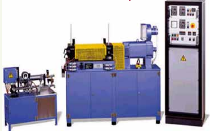
FZG Gear tester for Load Carrying capacity of Gear lubricants / Anti- Micropitting characteristics of gear oils
